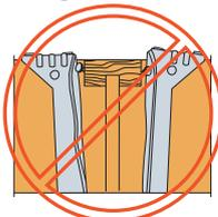
**Toenailing causes squeaks** and improper hanger installations. Do not toenail I-joists before installing top flange or face mount hangers.
