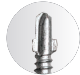
Wings to cut clearance hole means no sheet ride
