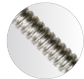
Annular threads (SCNR) create an interlock between the shank of the nail and the wood, providing superior holding power. Generally considered the nail type with the best withdrawal resistance.
